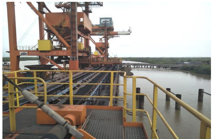
MULTIPURPOSE UNLOADERS, EACH FOR HANDLING OF 2500 TPH (IRON ORE), 1500 TPH (COAL & LIMESTONE) FROM 8000/10000 T BARGES & LOADING OF STEEL COILS (32 T, EACH) IN BARGES
