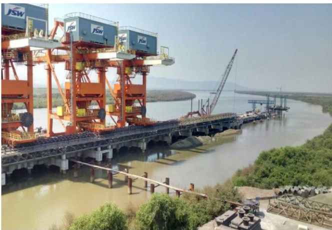
MULTIPURPOSE UNLOADERS, EACH FOR HANDLING OF 2500 TPH (IRON ORE), 1500 TPH (COAL & LIMESTONE) FROM 8000/10000 T BARGES & LOADING OF STEEL COILS (32 T, EACH) IN BARGES
